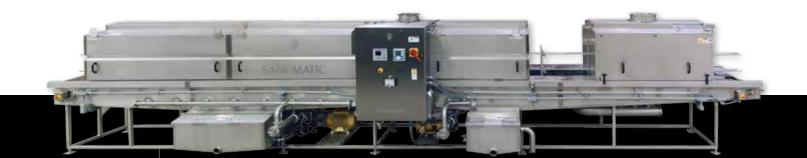
**The Sani-Matic Tunnel Wash** is an automated tunnel washer designed to clean a wide variety of high-volume items such as pans, totes, pails, buckets and trays. The basic design includes detergent and final rinse zones. Pre-rinse and recirculated rinse zones may be provided for heavy product residues or high-capacity requirements.
