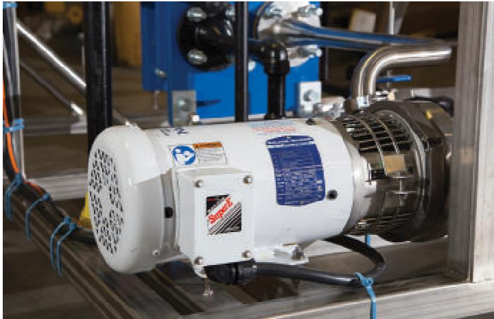
A centrifugal pump is part of a customized skid manufactured by M.G. Newell. JULIE KNIGHT/TRIAD BUSINESS JOURNAL
